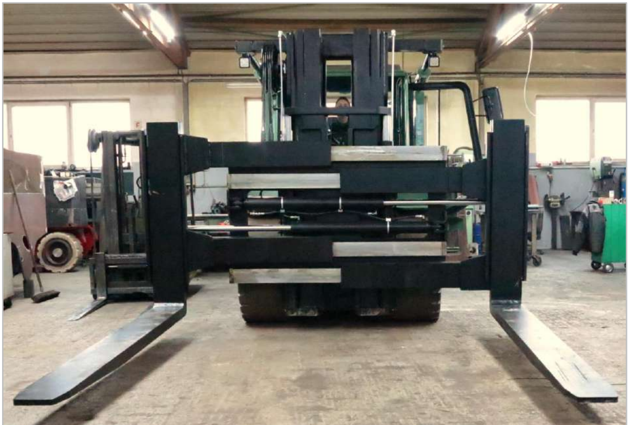
Maximum fork adjustment of a MKF 20 ton electric forklift
